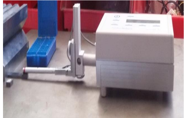
Fig. 4 Measurement of the surface roughness.
