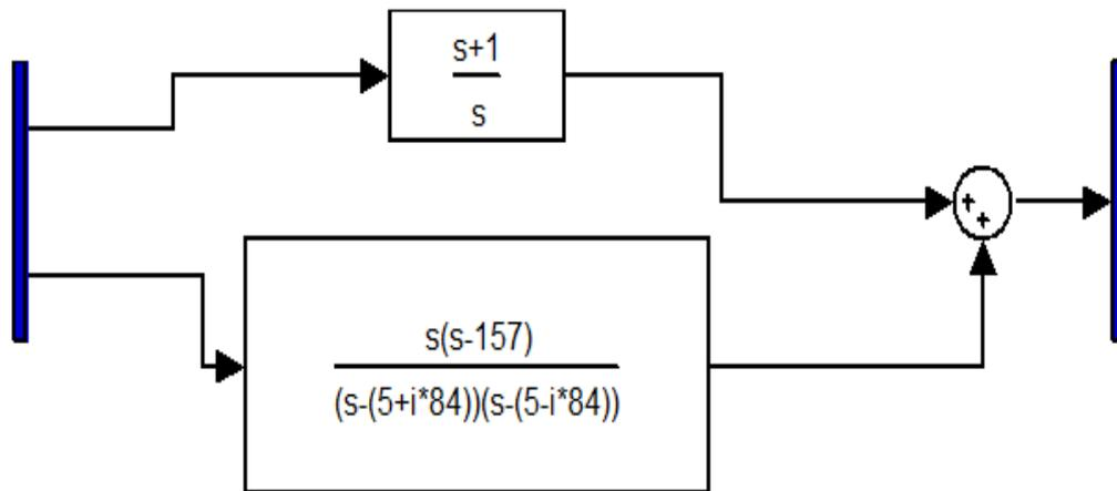
Fig. 1. Block diagram of VPI regulator.
