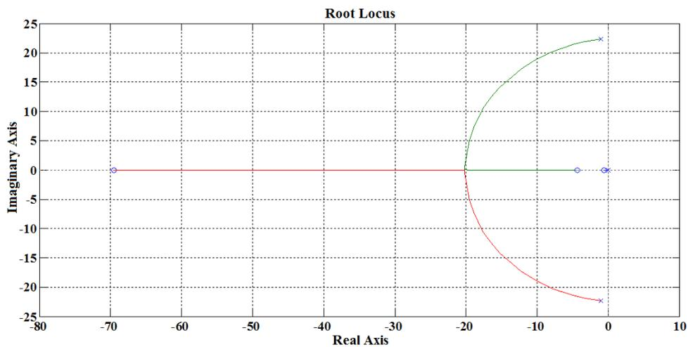
Fig. 3. Closed-loop locus of the VPI poles.
