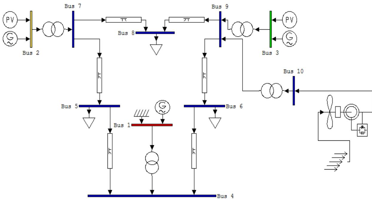
Fig. 13. The studied grid in the presence of DFIG.
