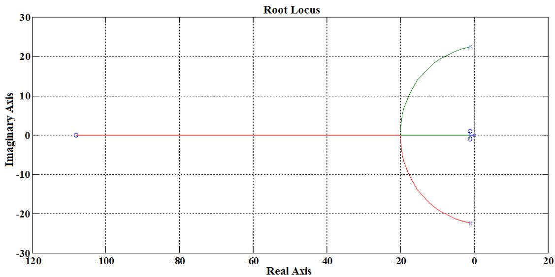
Fig. 2. Open-loop locus of the VPI poles.
