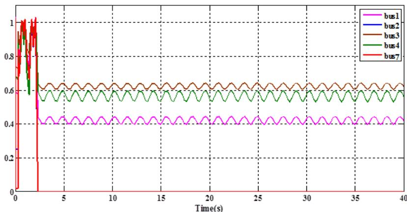
Fig. 9. Voltages of some buses in 0.25s fault.
