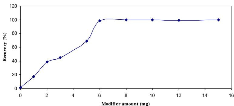
Figure 2. Percent recovery of 10 µg of Cu<sup>2+</sup> from an aqueous solution (250 mL) by the membrane disk at a flow-rate = 30 mL min<sup>-1</sup> at pH=4 washed by 10 mL of HNO<sub>3</sub> 3.0 M at a flow-rate = 10 mL min<sup>-1</sup> and varying amounts of BDSC.
