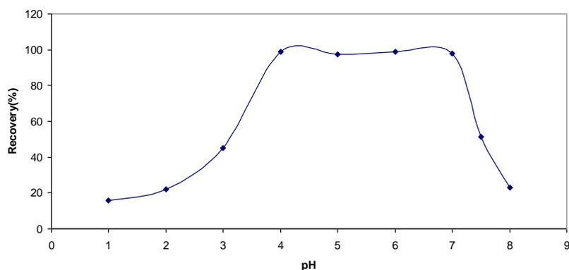
Figure 1. Effect of pH on the percent recovery of 10 µg of Cu<sup>2+</sup> from 250 mL aqueous solution by each C<sub>18</sub> disk impregnated with 6.0 mg of BDSC.
