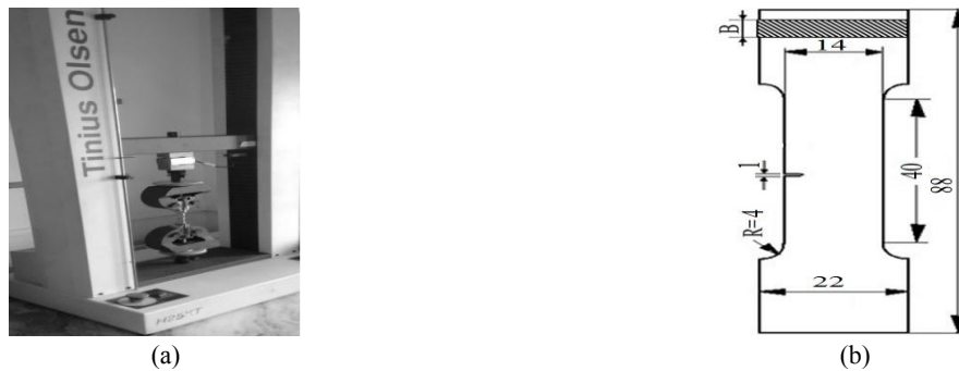
Fig.1 a) Specimen loaded on UTM. (b) Specimen as per ASTM standard.
