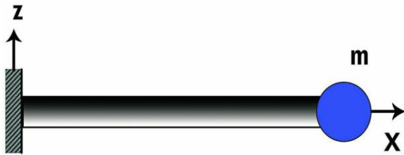
Fig.1 Geometry and coordinates of functionally graded cantilever Nano beam attached to a concentrated mass at the free end.
