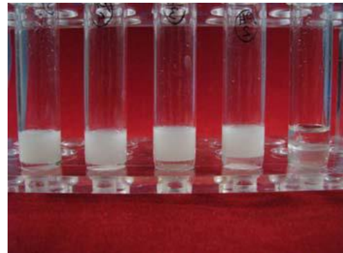
Figure 11. Forms A and B are the level of rhamnolipid emulsification at different pHs.
