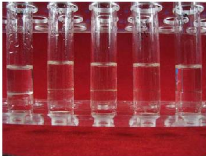
Figure 12. E24 rhamnolipid test at concentrations of 0.02, 0.04, 0.06, 0.08 and 0.1 g/l of sodium chloride.
